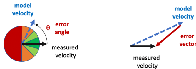
Fig.5: We compare both error angle (left) and Normalized Error Vector Amplitude (NEVA) (right) of measured surface currents (black arrow) with direction of the model forecast (blue arrow).
