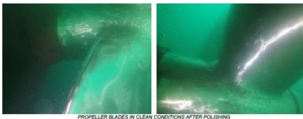
Fig.10: Pictures of the propeller after the propeller polishing
