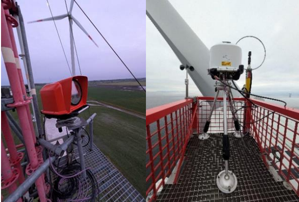
Fig.5a: Vaisala WindCube Nacelle (4-beam pulsed DBS type nacelle lidar)
