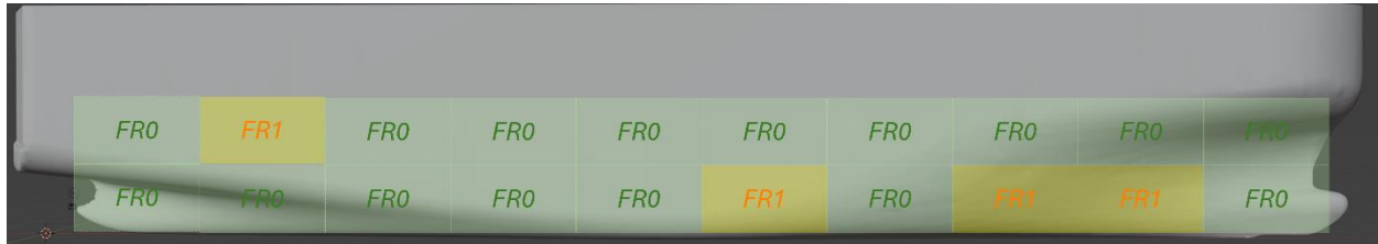
Fig.9: Vessel divided into sections and rated based on USN FR scale
