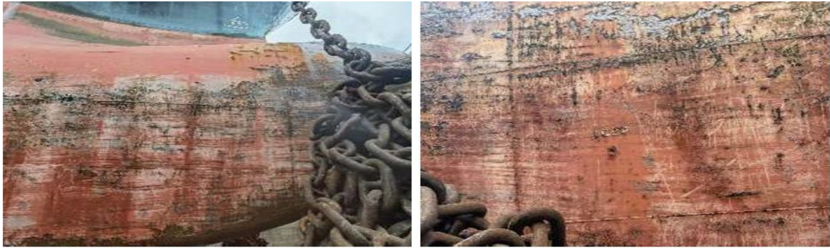
Fig.19: Photographs of the arrival condition of a container ship with ~10% animal fouling (Selektope-containing coating on flat bottom and vertical sides)
