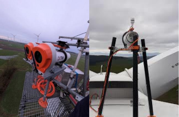
Fig.5b: ZXTM (continuous-wave VAD type nacelle lidar)
